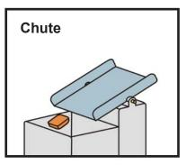
Use an up-and down flip plate to sort the product under test, suitable for bulk food.
