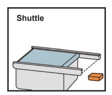
The push rod driven by the cylinder is used to sort the product under test, which is suitable for medium and large packaging products.
