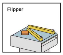
Use left and right swinging arm to sort the product under test, suitable for thicker products.
