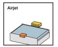
Use high pressure air to separate The push rod driven by the the tested products, suitable for light food or bulk food.
