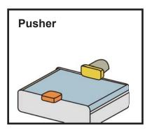
cylinder is used to sort the product under test, which is suitable for medium and large packaging products.
